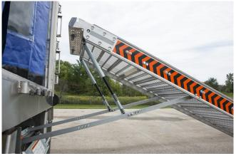
Two styles of lift assists are available – long and short, depending on the dimension from the enclosure to the trailer floor.
