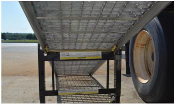
Double your ramp's life cycle with the ability to turn your panels over when one side wears down.
