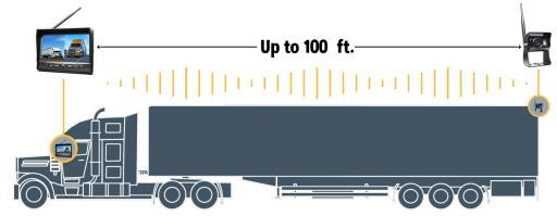
Our wireless camera systems boasts digital wireless range from 70 to 100 feet which is guaranteed to work at highway speeds. Installation takes less than an hour and the system comes with an instant pair feature which allows the driver to pair camera to monitor without leaving the cab.
