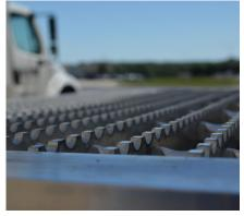
The serrated walk surface provides superior traction and with each step ice, snow mud and debris falls to the ground.
