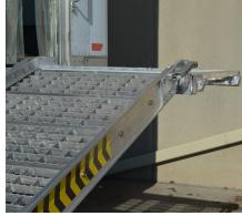
The design of the TSAP210A allows drivers to either attach a ramp to the platform or use the retractable ladder to access the trailer.
