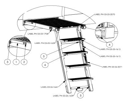
**IMPORTANT:** It is recommended that the platform stairs be used on a level surface. Be sure to regularly inspect your platform for loose fasteners, and repair or replace damaged parts. Any parts that are damaged or loose can cause serious injury. Improper usage of the platform can cause damage and possibly void any remaining warranty. Please contact your Territory Manager at 800-323-7424.
