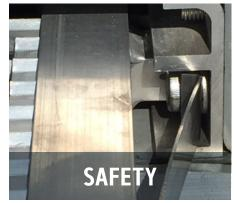
Spring lock ensures the FDP 3123L stays in place and disengages on your command.
