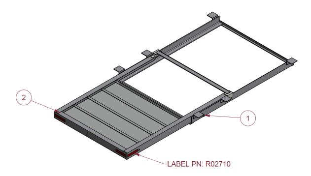
**IMPORTANT**: R•O•M also recommends that the platform be used on a level surface. Be sure to regularly inspect your platform for loose fasteners, and repair or replace damaged parts. Any parts that are damaged or loose can cause serious injury. Improper usage of the platform can cause damage and possibly void any remaining warranty. Please contact your Customer Development Representative at 800-827-3692.
