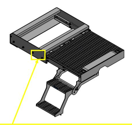
Serial number located on the front left corner of the platform
