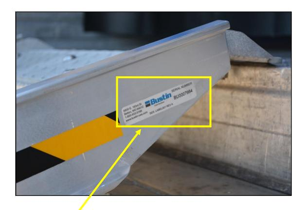
Serial number located on the top outside of right rail
