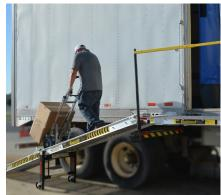
With a 2,000 lbs. capacity drivers can attach a ramp to the platform or use the portable ladder to access the trailer.
