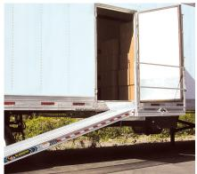
A ramp can be attached to the platform to run perpendicular to the trailer to avoid running into traffic.
