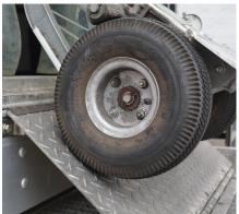
The hinged down mini-ramp makes it easy to transition from the trailer floor to the platform.
